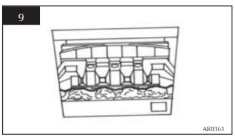
• Put five of the round coals on the front between the fingers of the flame baffle.
